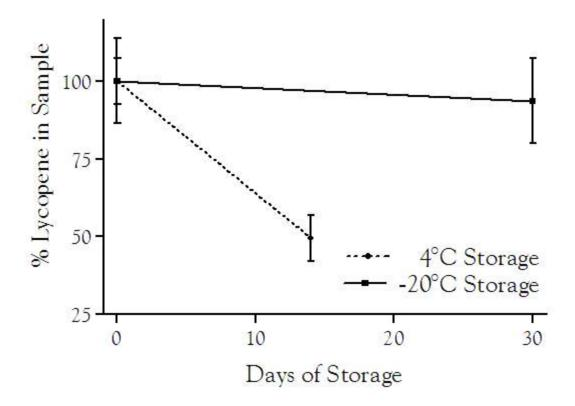
Figure 3.2 Stability of lycopene in freeze-dried tomato powder over time at -20°C and 4°C. Degradation was not significant after 30 days at -20°C (p=0.1531, n=12), but was highly significant after 14 days at 4°C (p<0.005, n=12).
